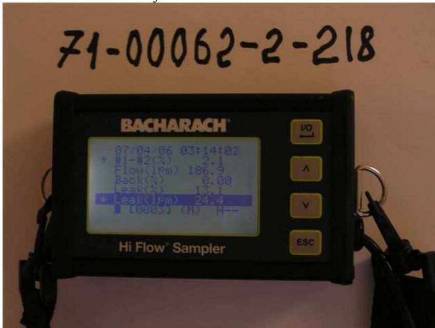
Picture 3 Measurement of leak rate
